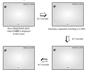
Automatic sequential switching to CAM5
